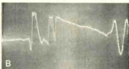
Figure 5 —Trace expansion: The original trace as captured in A, is expanded in B to view transients that occurred immediately after triggering, left.
