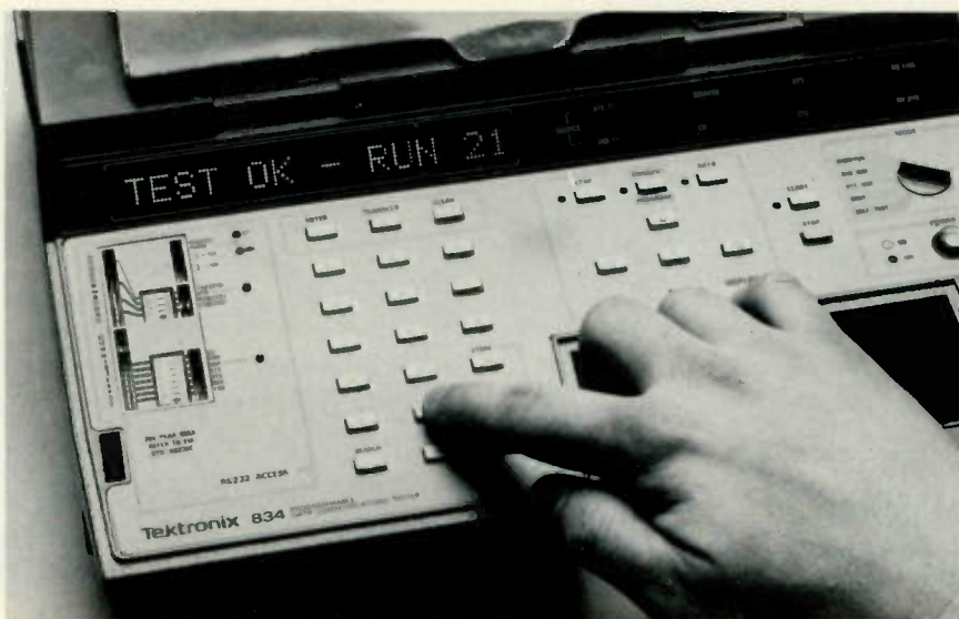
Figure 3 The Tektronix 834 Programmable Data Communications Tester.
