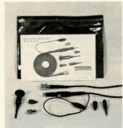
Figure 4 A scope-type low-capacitance probe (such as this SP-7 Hickok probe) is required for proper operation of the Logi-Track function.
