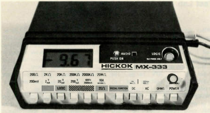
Figure 1 Hickok model MX-333 has all standard DMM features and 0.1% basic dcV accuracy, Vari-Pitch audio indication of the reading, Logi-Track indications of pulses and supply voltages, a 20 \Omega low-resistance range and an effective diode test.
