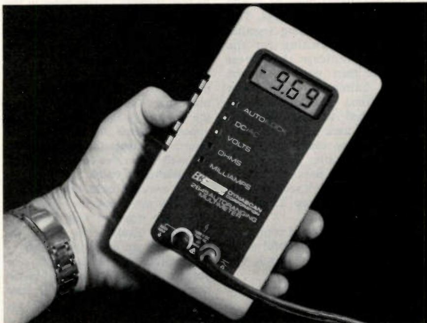
Figure 1 B&K-Precision model 2845 3½-digit LCD-readout multimeter features computer-controlled autoranging and 0.1% dcV accuracy. Function pushbuttons are side mounted for convenient hand-held operation. Indicators show switch positions. Only two test-lead jacks are needed. All functions are protected from damage by overloads.
