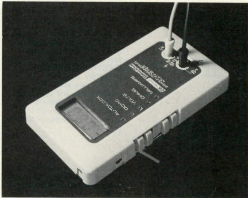
Figure 2 A plastic tilt stand is attached for bench operation. The stand can be moved so it becomes a bail for hanging the multimeter. Autoranging makes possible efficient operation with just a few push-buttons and two test-lead jacks. One on/off switch and five push-buttons (one left side) are the only controls.
