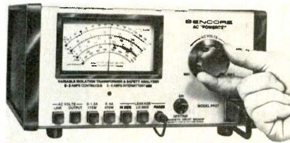
Figure 1 Sencore AC Powerite model PR-57 performs four functions for ac line power. It is a variable-voltage isolation transformer with meter read-outs of voltage, current and wattage, plus a convenient and accurate safety leakage test.
