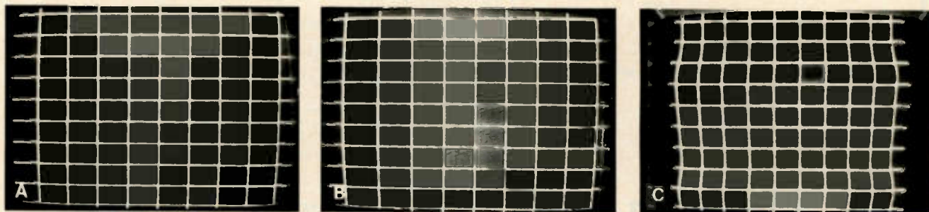
Figure 1 Crosshatch patterns reveal many horizontal defects. (A) This is the normal crosshatch for comparison. (B) A shorted L106 linearity coil expanded the linearity at the left. (C) When SCR100 regulator was shorted, shut-down occurred at normal line voltage. After the line voltage was reduced to about 90V, a small raster with 120Hz hum could be seen.
