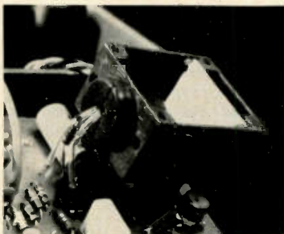
Photo (A) shows the phototransistor end of the beam-splitting mirror. (B) The infrared LED is on the chassis below the mirror assembly.
