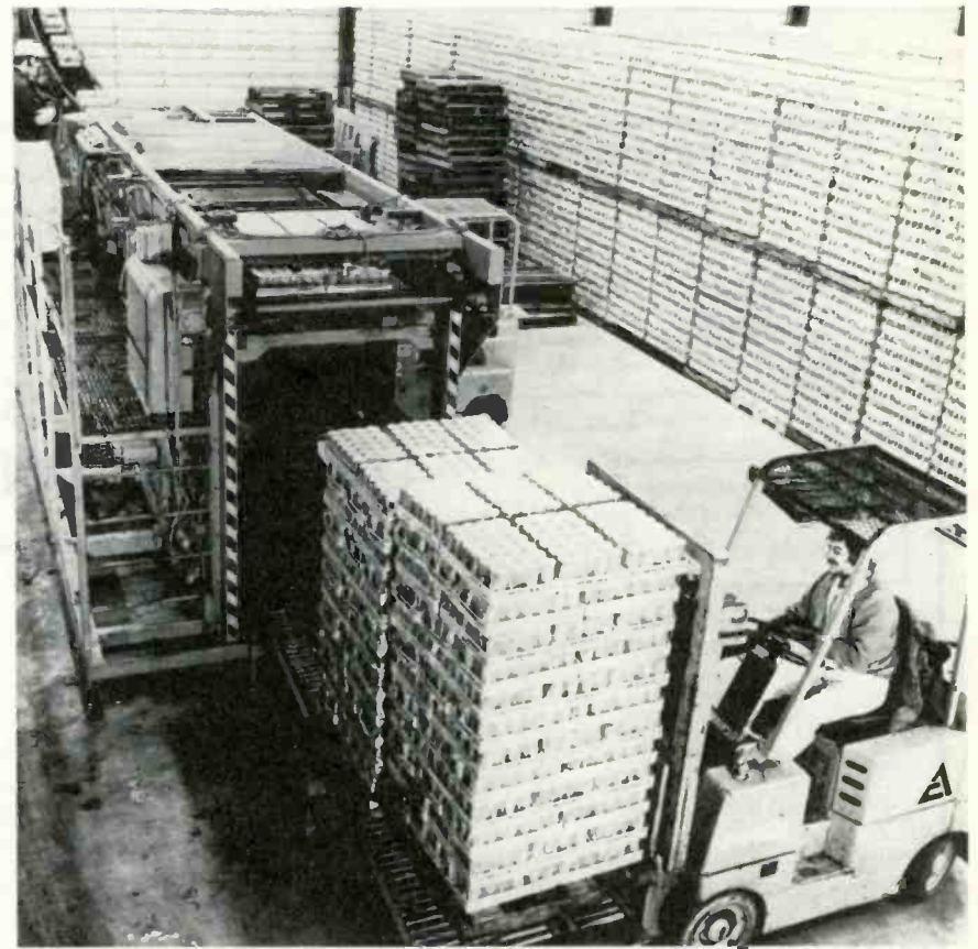
Production of this palletizer (shown supplying a high-loader) was increased by 25% in one Coca Cola plant when an older controller that used relays was replaced by a programmable electronic controller. Faster operation was possible without the relay-cycling time delays. Photos courtesy of Struthers-Dunn.
