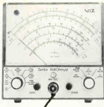
Typical of VTVMs and FET-meters is this VoltOhmyst. (Courtesy of VIZ)
