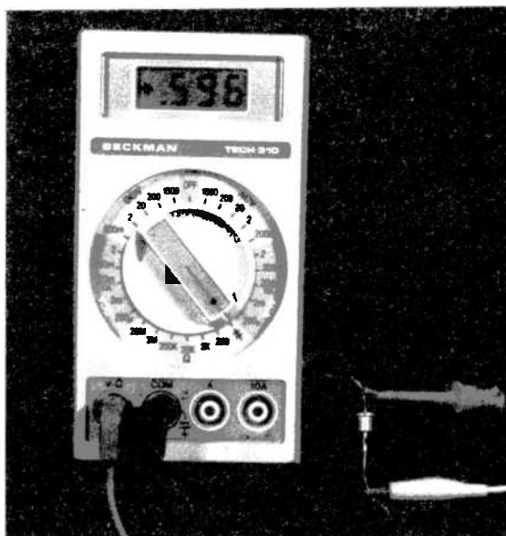
Overrange indication is a non-flashing "OL" as shown.
