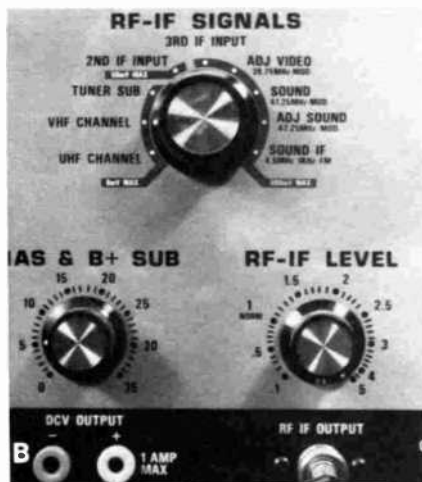
Figure 1 RF and IF signals for signal injection tests of TVs are regulated by these controls.
