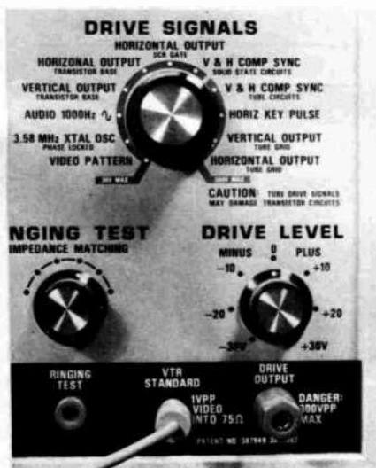
Figure 11 Waveforms for signal substitution in sync, sweep, audio, chroma or video are selected by the "Drive Signals" switch. Signal amplitude and polarity both are adjusted by the "Drive Level" control. Then the selected signal emerges from the "Drive Output" jack.
