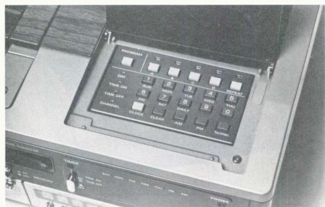
General Electric's 4-hour programmable VHS videocassette recorder permits recording of five programs at different times on five days during one week. The user follows the reminder lights for step-by-step programming.
