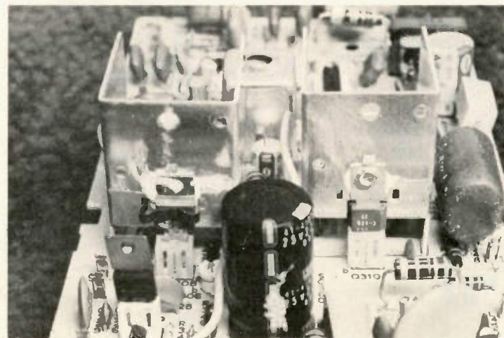
This view of the deflection module after removal from the chassis shows many of the vertical components. The power transistor at the lower left is Q304, the driver. Both output transistors are mounted on large aluminum heat sinks. Q308 is at the left, and Q310 is at the right. The transistors plug into sockets, and the heat sinks come out with the transistors. Just squeeze the two top front edges of the heat sink towards each other, tilt up the front part of the heat sink (to release the catches) and the heat sink with transistor easily lifts out. Evidently, these outputs come from different sources, for one was mounted by a screw, and the other of a different shape was mounted by a metal spring. The heat sinks are connected to the collectors, making fine test points. The black part at the lower center is the output capacitor C344. All of the solid-state components of the vertical circuit are mounted in sockets for easier servicing.
