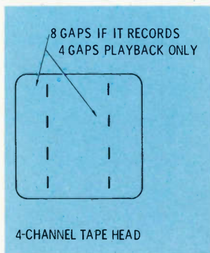
Figure 2 Four gaps (each with internal core and windings) are required for a head to give four-channel stereo sound. Four additional gaps are necessary for erasing, if the machine also records tapes.
