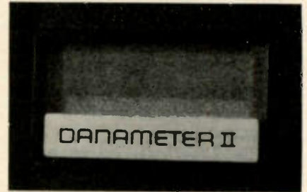
Figure 2 The black digits of the Danameter appear to be formed on clear plastic at a short distance from the backing. Brighter room lights increase the brilliance of the diffused reflector which is behind the black digits. One picture shows the battery-test display; the other is the display, but with the meter turned off.
