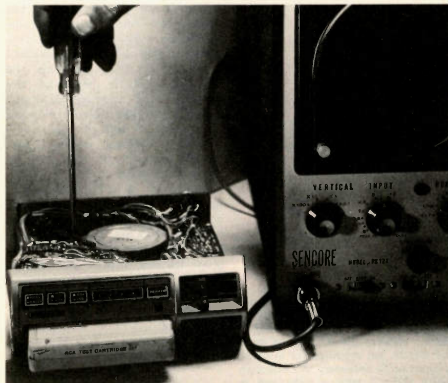
Figure 5 A test cartridge is strongly recommended for tilt and elevation adjustments, along with a scope as the indicator. A meter or a listening test can be used, but tape hiss and noise reduce the accuracy.
