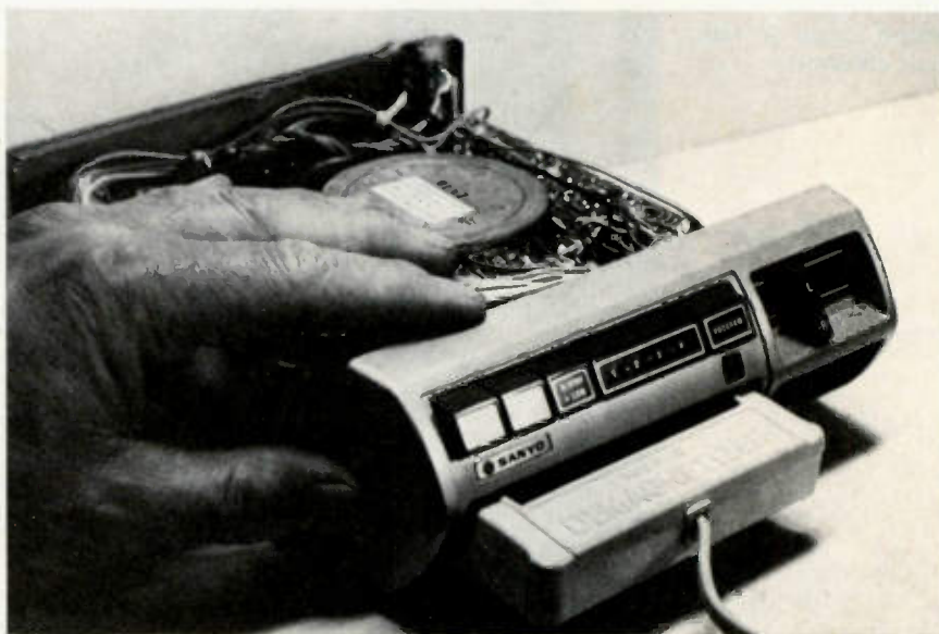
Figure 3 Tape heads should be demagnetized often. Use a long degausser, or insert a special demagnetizer Stereo-8 cartridge. With conventional demagnetizers, take care to not scratch the face of the head.
