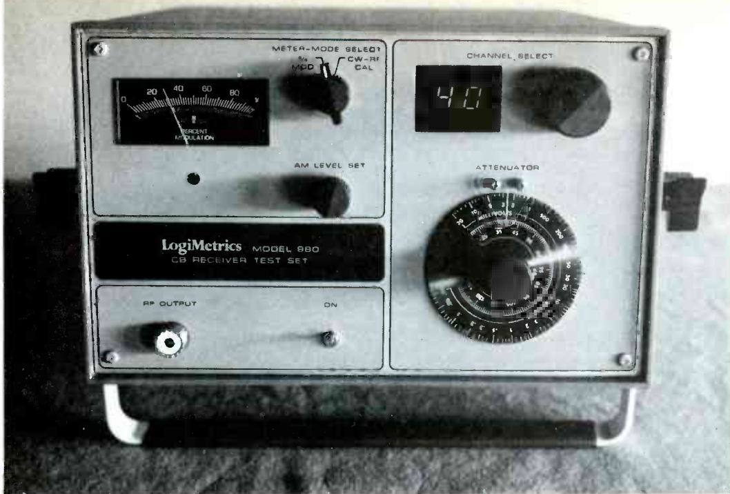
Fig. 1 Model 980 CB-receiver generator by LogiMetrics features accuracy and simple controls, made possible by sophisticated digital circuits.
