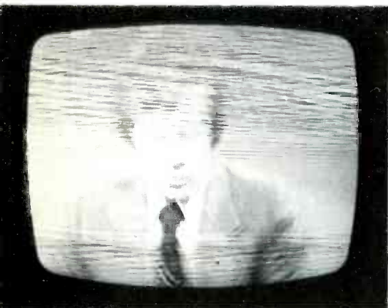
Fig. 1 Where should you look for the cause of this peculiar picture: vertical, horizontal, pincushioning, AGC, or power-supply hum?
