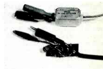
Fig. 1 In order to produce curves that are truthful, it is absolutely necessary to use proper pads and probes with the sweep equipment. At the top is the 39G26 Sencore quadrupler link detector, and a similar home-made quadrupler is shown at the bottom.
