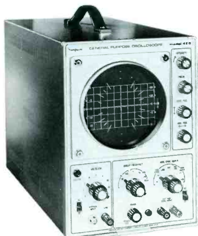
Fig. 1 This is the Simpson Model 455 general-purpose 5-inch scope.
