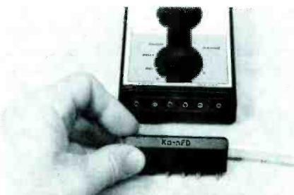
Fig. 10 At the meter end of the wires to the press-to-read probe is the large plug which must be turned one direction for volts and reversed for capacitance and resistance readings. The extra two prongs at the center are for the remote switch in the probe.
