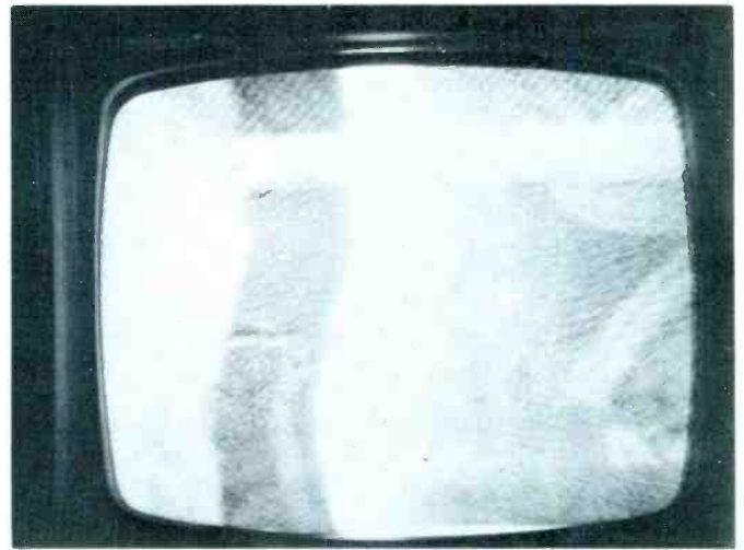
Fig. 5 In extreme cases of cross-modulation distortion, the blanking bars of another channel can be seen along with the normal picture. The effect is exaggerated here because the video of the desired channel faded out between scenes. Less severe overload makes the picture look grainy.
