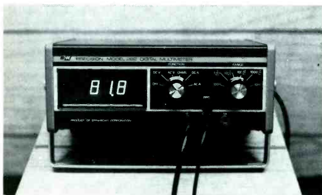
The B&K Precision Model 282 DMM has the ranges most needed for testing home-entertainment electronic products. Some of the features are a 3-1/2-digit Sperry display, auto-polarity, and shielded test leads.
