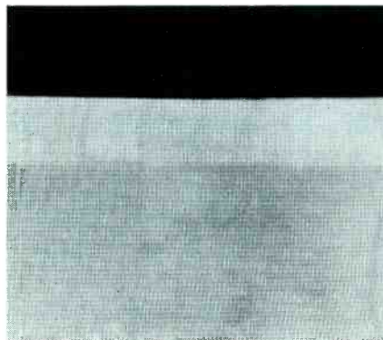
Fig. 4 At top of the screen is what appears to be a half scanning line. However, scope waveforms (picture at right) show it is produced by blanking, not scanning.
