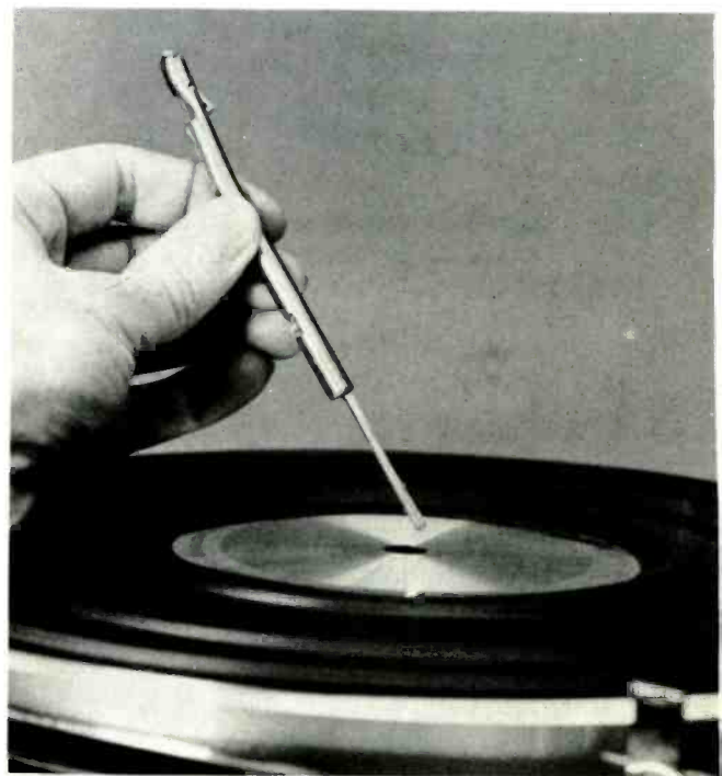
Step 9 This spindle is removable—as are most turntable spindles—and has a long activator rod. Movement of the activator rod is sideways, moving the pushoff tab out and back, and then a little further until it protrudes in the other direction. This far-forward motion senses any more records on the stack; if none, the machine shuts off after the record that just dropped has played.
