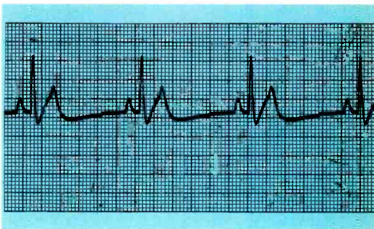
(B) Sample of an actual ECG waveform on paper tape from a strip-chart recorder.
