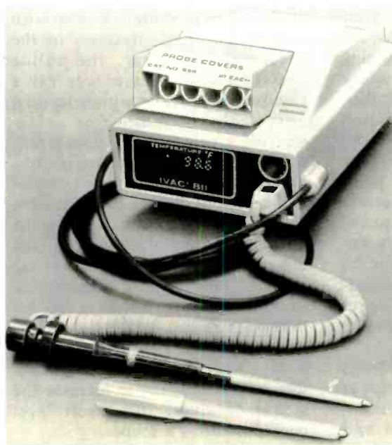
Fig. 11 Portable electronic thermometer (IVAC Model 811) uses a thermister inside a disposable tip. The thermister is in a bridge circuit, and any unbalance is displayed by the digital readout. (Courtesy of IVAC Corp.)
