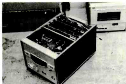
Fig. 8 Top view of the Model 7807C Hewlett-Packard heart-rate meter. The meter on front has a long, horizontal, analog scale. Complexity of the circuit is shown by the several plug-in circuit boards.
