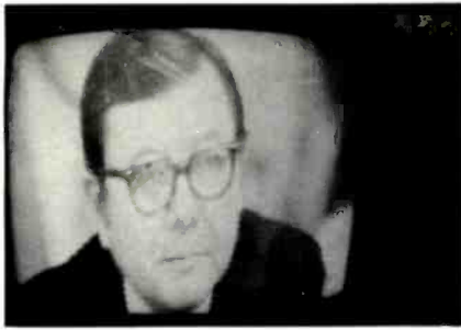
Fig. 10 Narrow width at the bottom, and some horizontal displacement of scanning lines appeared on this Zenith 20CC50.
