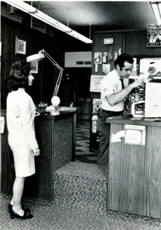
Fig. 3 A carry-in service counter has all the equipment necessary for most repairs. Minor repairs are made as the customer waits. Notice the low lift-through section of the counter which is carpeted to avoid scratching portable television sets.
