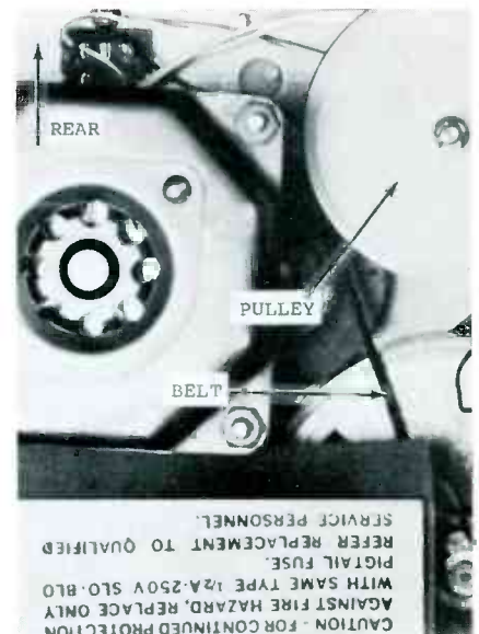
(B) But the large, white, felt wheel turns only so long as the takeup spindle turns.
