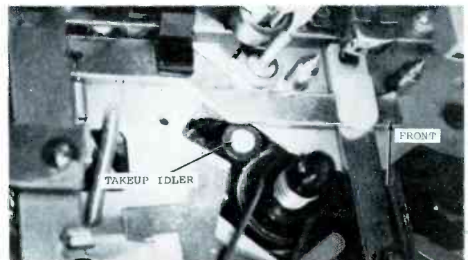
(C) This picture shows the take-up idler which was not included in Fig. 1.
