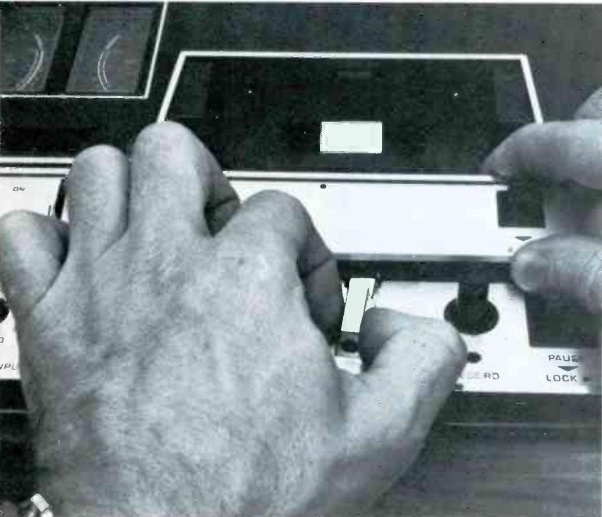
(C) Hold the Rewind/Fast-forward knob forward while you lower the top, then align it so the set screw fits the handle.
