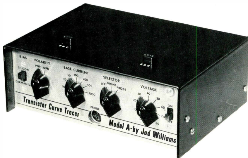
Fig. 1 Jud Williams Model A transistor curve tracer, one of at least three commercially produced curve tracers now available. Unit shown here simultaneously applies one step of a staircase waveform of current to the base of a transistor and a parabolic voltage to its collector. Emitter-collector current (voltage dropped across emitter resistor) is used to drive the vertical deflection of a scope and the collector voltage provides horizontal deflection. The resultant waveform is a "family of curves" which reveals the degree of control the base exercises over emitter-collector current, levels of leakage between junctions and AC gain, or beta (ratio of base and collector currents). Two three-prong sockets on top of unit are for out-of-circuit testing of transistors. Three-prong probe which is plugged into PROBE socket on front panel of unit is used for in-circuit testing. Connections to scope are located at rear of unit.
