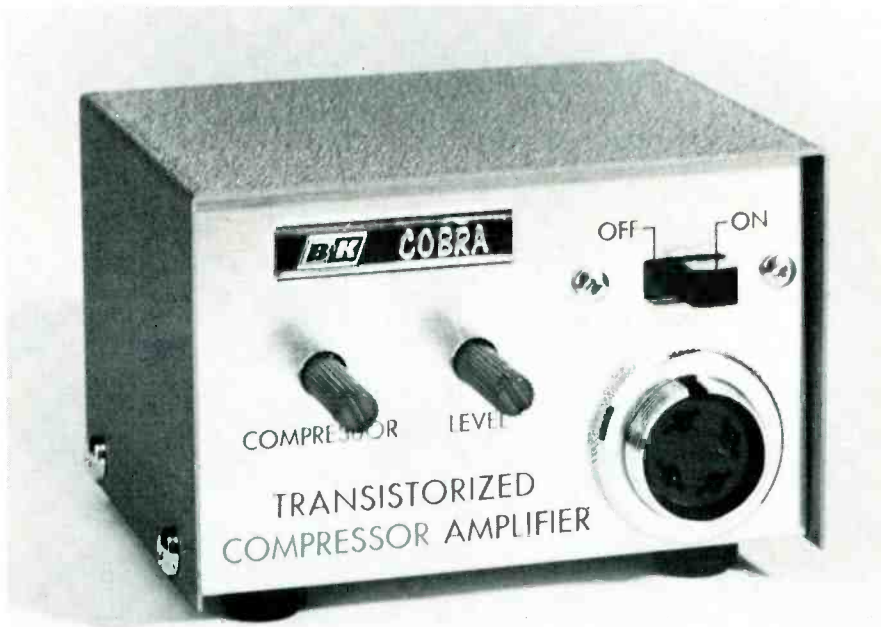
Fig. 4 Two knobs on this compressor/expander type of modulation controller can be turned by operator—not a good idea, because scope and modulation monitor are needed for optimum adjustment.
