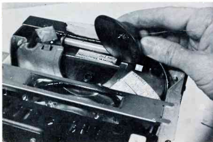
Fig. 8 Circuitry surrounding Trinitron picture tube stresses simplicity, compared with shadow-mask-tube circuits. Photo shows second-anode cap at top of tube instead of at side of bell as in conventional CRT's.
