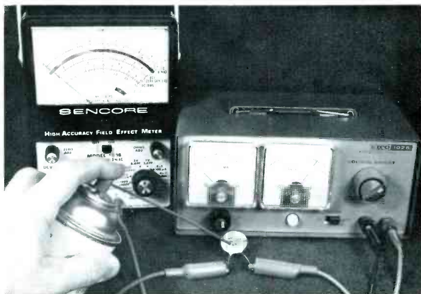
Fig. 1 Test setup shown here is for checking leakage of capacitor with low voltage rating. Leakage is indicated in form of voltage by FET VOM. If leakage drastically decreases when capacitor is sprayed with coolant, defect is heat sensitive, or thermally intermittent. Plastic tube attached to nozzle of can enables the technician to confine the coolant to one component or small area of circuit.
