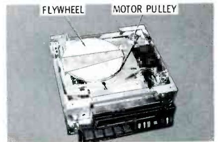
B) Combination AM-FM multiplex radio and stereo tape player made by Phillips of Canada for Chrysler. Parts and warranty are handled in U.S. by Bendix.
