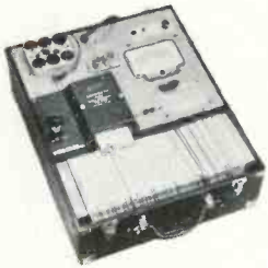
123R CARDMATIC TUBE TESTER —Automatic tube testing using card-programmed switch, eliminates errors. A fast, automatic tube tester which includes tests for saturation and cut-off in addition to mutual conductance.
