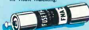
FNA FUSETRON Fuse 13/32 x 1 1/2 in. slow-blowing, Visual-Indicating, Alarm-Activating. (Also useful for small motors, solenoids, transformers in machine tool industry.)
