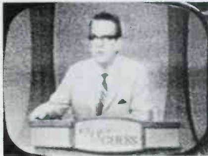
Fig. 7 Snow in picture is common indication of tuner trouble. Above, A, Heavy snow caused by weak RF tube or defective balun. Below, B, Medium snow resulting from slightly weak RF tube, noisy transistor, or AGC trouble.
