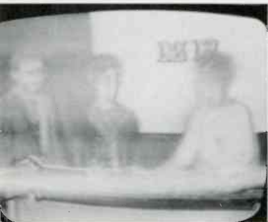
Example of trouble symptom displayed by a defective color CRT. Smeared and improperly focused picture was caused by a shorted picture tube.
