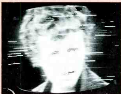
Fig. 2 Less severe case of motor-noise from electric shaver.
