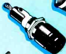
HPC Panel mounted holder for 13/32 x 1 1/4 in. fuses. Rated 30 amperes for any voltage up to 600.
