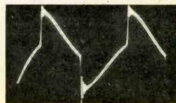
Fig. 26. Differentiation, ringing, and overshoot in a square wave.
