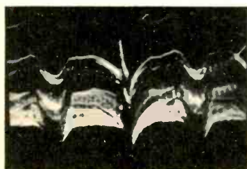
Fig. 13. Hum in the video-IF signal.
