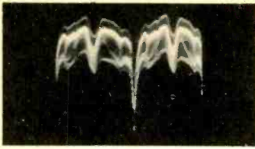
Fig. 6. Typical pattern obtained in an IF signal-tracing test.
