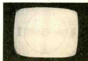
Fig. 15. Picture has low contrast.
