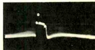
Fig. 22. Video signal with white portions compressed.
