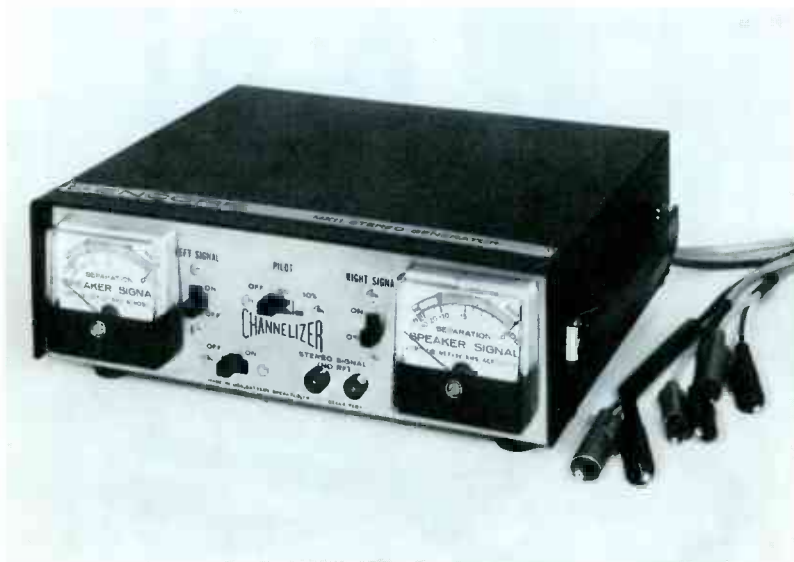
Figure 4. New light-weight MPX generator.
