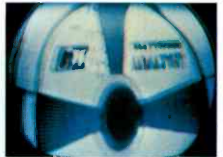
Fig. 6. Clod pulled the vertical linearity up until the raster filled the screen—the heck with linearity!
