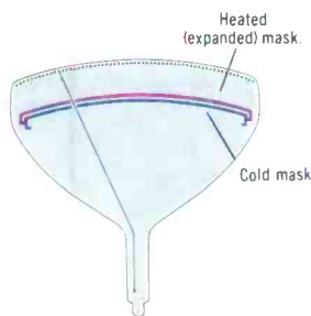
RCA Hi-Lite tube with Perma-Chrome . Exaggerated drawing shows locked-in register of beam with phosphor dot as shadow mask is heated. NOTE: Mask moves toward face of tube as it expands. Apertures in shadow mask move along paths of electron beam as mask expands or contracts with rise and fall of tube temperature.
