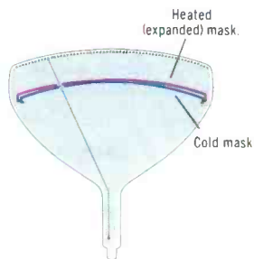
Brand "X" tube without Perma-Chrome . Exaggerated drawing of cross-section of rectangular Brand "X" tube shows the expansion of the shadow mask and the change in beam-landing register.
