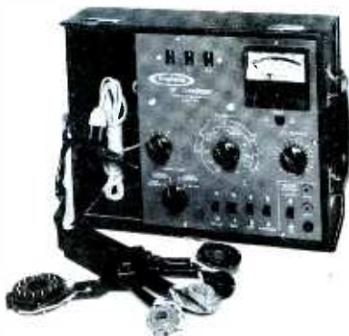
Fig. 1. CRT tester has KV meter.
