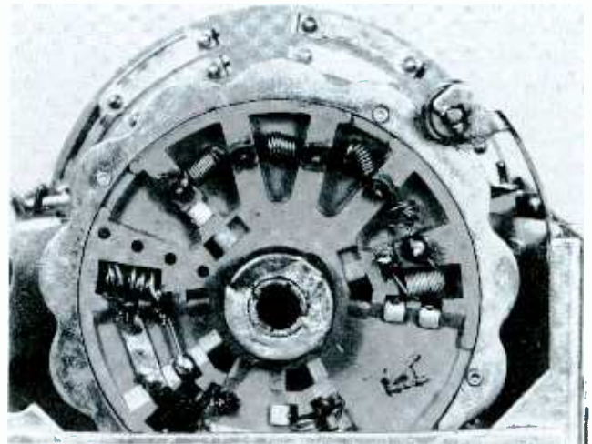
2 Fig. 2. Less frequently, looseness develops in the rear shaft. The looseness appears between the shaft and the odd-shaped brass washer, or between the washer and the disc. Test the rear disc for looseness.
