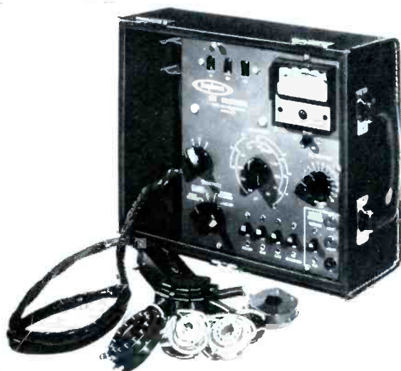
Compact and only 7½ lbs, the CRT Commander has a built-in high impedance voltmeter (so you don't have to carry a VTVM). Price: $89.95.
