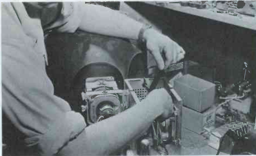
Fig. 7. Example of wrapping the high-voltage lead to prolong circuit life.
