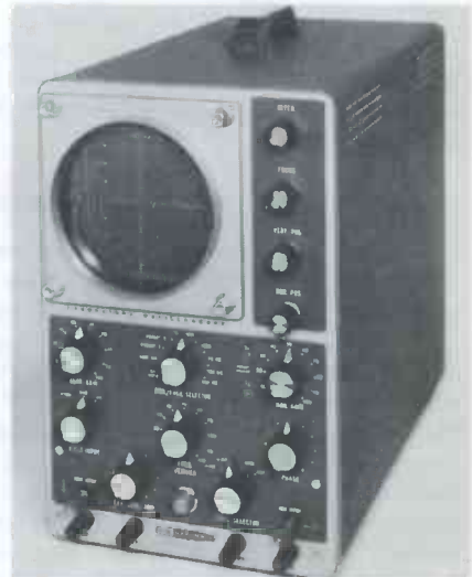
Fig. 1. 5-mc scope has front-panel adjustment for two preset sweep freqs.
