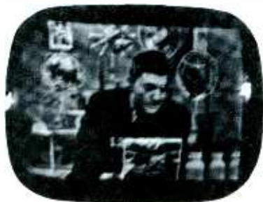
Fig. 1. Raster is reduced in size in both directions due to defective power-supply rectifier.
