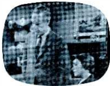
Fig. 5. Typical case of mild raster shrinkage depicted here may not show on all stations.
