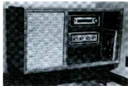
Fig. 8. Discarded TV cabinet converted into an FM-Phono stereo hi-fi home music center.
