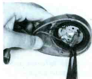
Fig. 4. To remove cartridge, remove C-ring.
