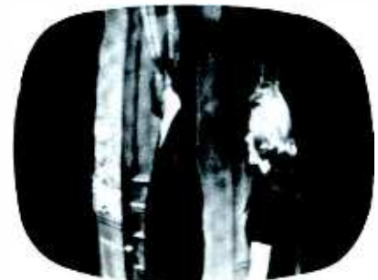
Fig. 10. Shrinkage of raster resulted from unnoticed shift in width-adjustment control.
