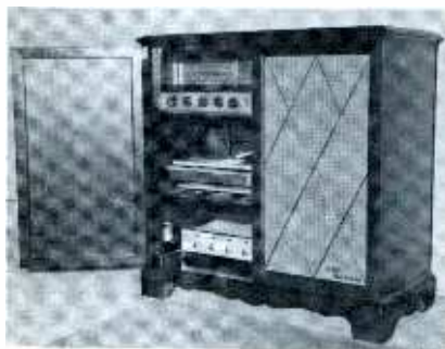
Fig. 1. The phono console shown here was monophonic, but was converted to stereo.
