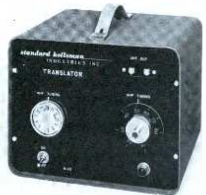
Fig. 8. Translator provides signals on UHF channels from the signals of VHF stations.
