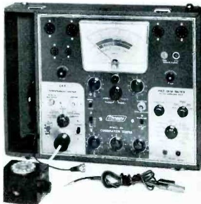
Fig. 7. A combination tester providing functions of VOM, tube tester, CRT rejuvenator.
