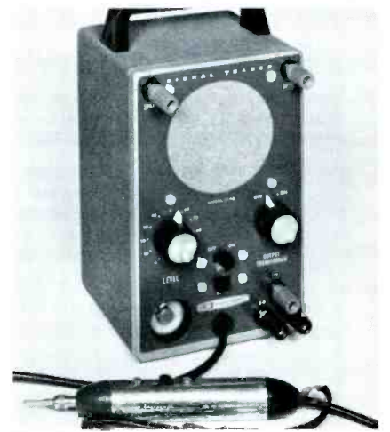
Fig. 3. Signal tracer includes a noise-test function and has aural and visual indication.
