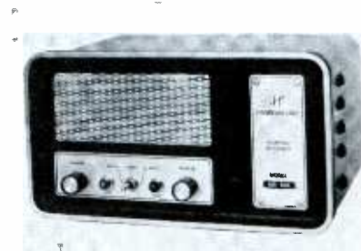
Fig. 1. Fixed radio paging receiver equipped with tone decoder of type shown in Fig. 4.
