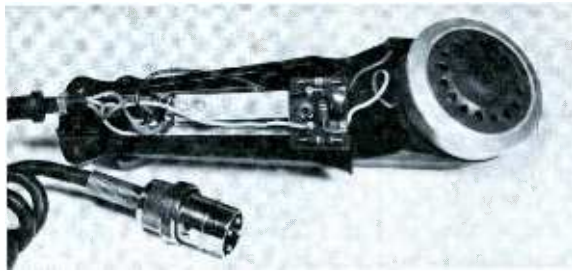
Fig. 8. Transistorized microphone has printed circuit board.
