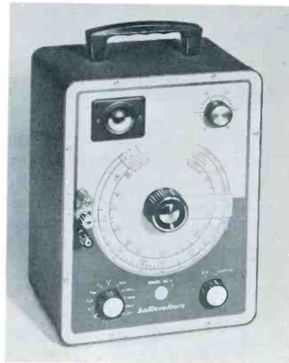
Fig. 2. Capacitor testers subject the capacitor to stress encountered in the circuit.
