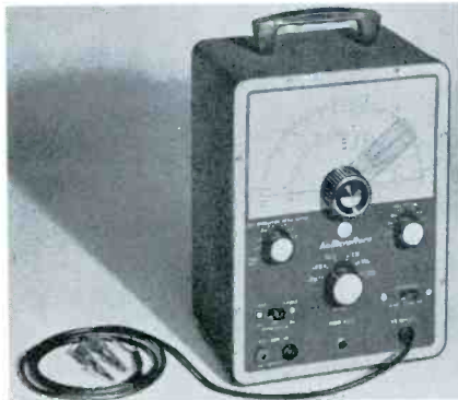
Fig. 15. This generator provides modulated RF or CW from 50 kc to 220 mc in 8 ranges.
