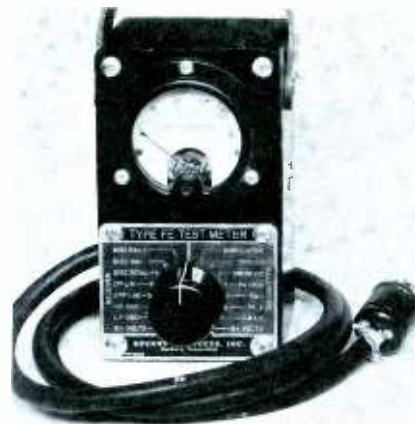
Fig. 5. A meter to be plugged into the several test receptacles on mobile two-way radios.
