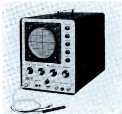
Fig. 9. A direct reading wideband scope is useful for either monochrome or color TV.
