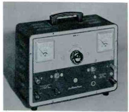
Fig. 11. Variable DC supply can be used for transistor radios if ripple is low enough.
