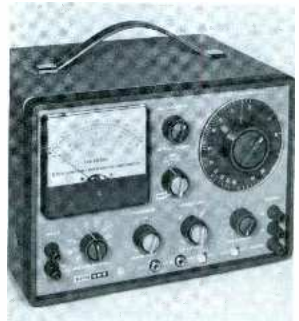
Fig. 4. Distortion meter and AC VTVM features well planned layout of the controls. Instrument so that you can determine the exact power output delivered by an amplifier into all standard impedances from 3.2 to 600 ohms, from 1 mw to 100 watts.
