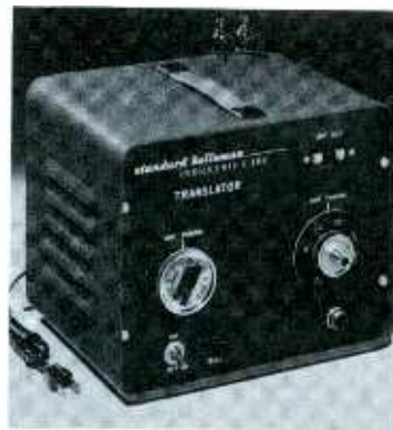
Fig. 16. This instrument generates UHF signals from VHF TV signals.
