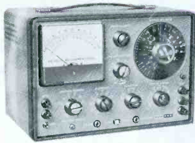
Fig. 13. Comparator determines the value of unknown resistance, capacitance, inductance, and milliammeter ranges from .01 ua to 15 ma.
