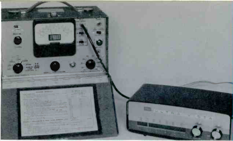
If your VHF FSM isn't easily convertible, connect the UHF antenna to a UHF-to-VHF converter and the converter output to the VHF FSM.
