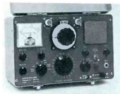
Fig. 4. Portable, multichannel frequency meters like this are excellent for field service.
