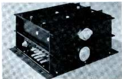
Fig. 10. A 275 watt power converter with a drop of only 8% from no load to full load.
