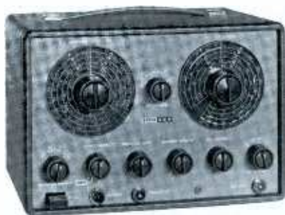
Fig. 19. A 4.5 mc crystal is provided with this instrument to align TV sound circuits.
