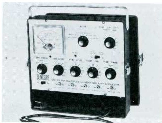
Fig. 18. Multiplexing generator with a P-P voltage and decibel meter.
