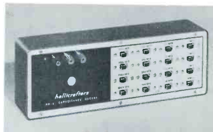
Fig. 1. A capacitance decade box aids in the location of suspected defective capacitors.
