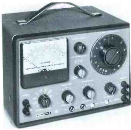
Fig. 5. This distortion meter is also AC vacuum-tube voltmeter and decibel meter.
