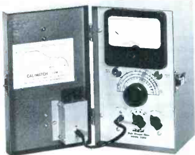
Fig. 6. A field-strength meter for measuring the strength of any VHF or UHF carrier.
