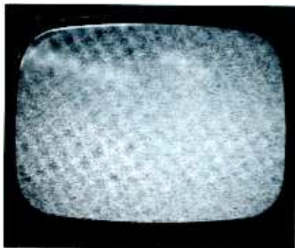
Fig. 1. Snow when IF stages are at high gain.
