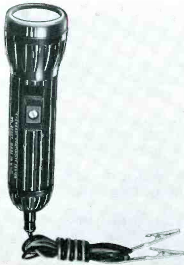
Fig. 4. A combination flashlight-continuity tester serves dual role for the technician.
