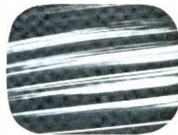
(A) Oscillator frequency low
