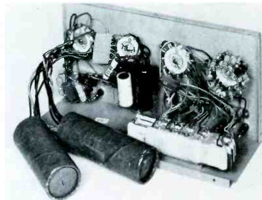
Fig. 4. Instrument substitutes for almost any part encountered in most electronic equipment.
