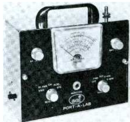
Fig. 1. Chrome-finished case houses several instruments for servicing CB transmitter.
