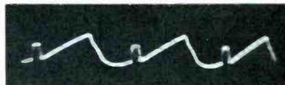
Fig. 5. Grid waveform of AFC stage corresponding to visual symptom shown in Fig. 4D.
