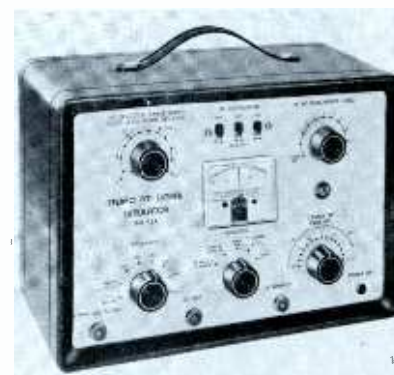
Fig. 1. Stereo FM signal generator can be used for sweep alignment of RF, IF.
