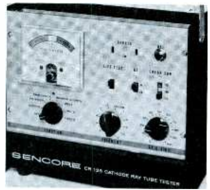
Fig. 7. New instrument is capable of rejuvenating color guns, one at a time.
