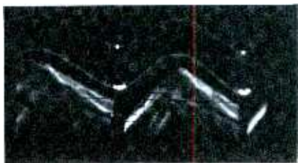
Fig. 9. Billowed raster was obviously a result of 60-cps hum in the video.
