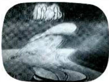
Fig. 1. Extreme twist due to cathode-filament short in a video IF tube.
