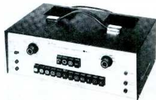
Fig. 1. Push buttons are distinctive features of this color-bar generator.
