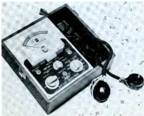
Fig. 1. New unit reactivates weak CRT's and, in some, even eliminates shorts.
