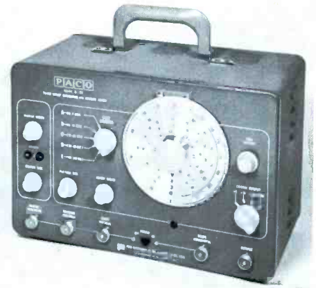
Fig. 3. Sweep generator includes self-contained marker adder for versatility.
