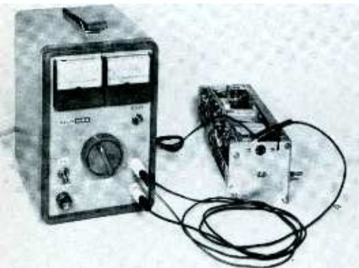
Fig. 1. The EICO 1064 operates DC-powered radios and charges batteries.
