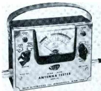
Fig. 5. Seco 520 measures power and SWR in transmitter antenna circuits.
