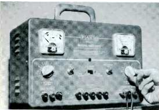
Fig. 1. Paco offers regulated, variable-voltage power supply in kit form.
