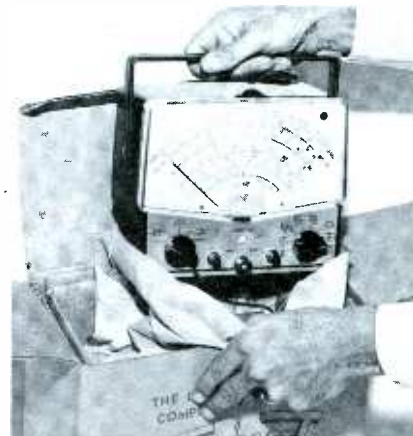
Fig. 5. Meter face covers two-thirds of front panel in Triplet Model 850.
