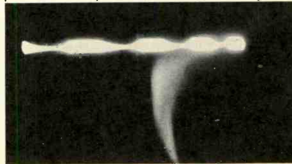
Fig. 9. Heater-to-cathode leakage occurring in cathode-ray tube commonly causes intensity modulation of the trace.
