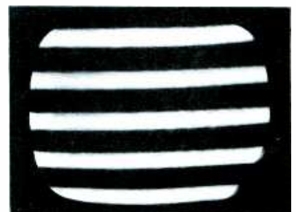
Fig. 2. Bars show on CRT when a sweep-generator signal is getting through.
