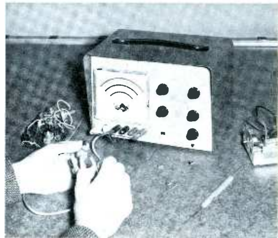
Fig. 4. Win-Tronix unit is designed for testing and analyzing transistors.
