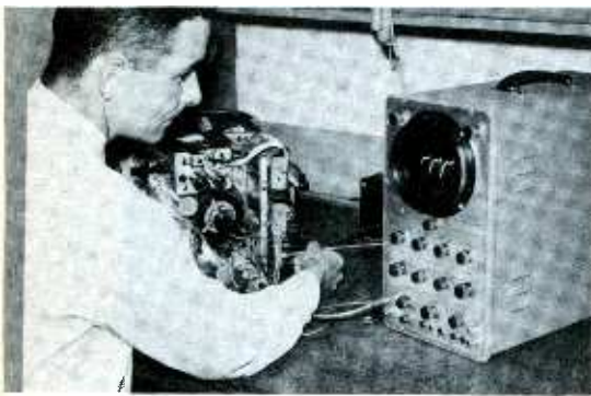
Fig. 1. Precision scope being used to align a horizontal sweep oscillator.
