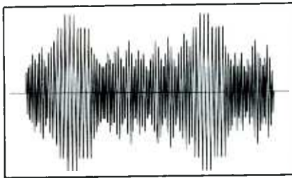
Fig. 7. Theoretical waveshape of modulated IF signal applied to detector.
