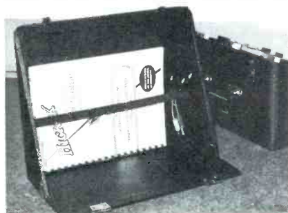
Fig. 5. The tester's detachable lid is used to store manual and test leads.
