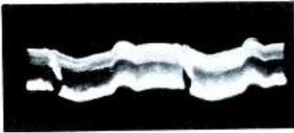
(A) Normal waveform obtained when probe is connected to plate of the final IF.
