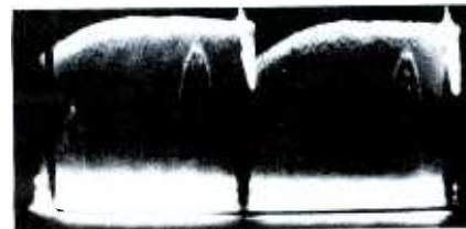
(D) Overdriven IF produced video detection at grid, as this waveform shows. Fig. 5. A low-capacitance probe can be used to check the final video IF stage.
