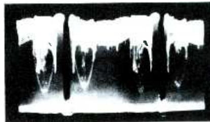
(B) When R8 is 10K, setting contrast at minimum produces this waveform.
