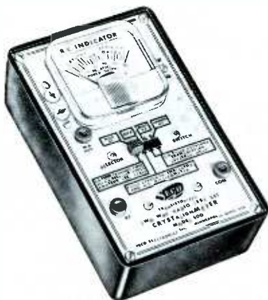
Fig. 1. Seco's new portable unit for checking Citizens band transceivers.
