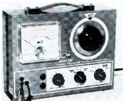
Fig. 1. B & K's new two-in-one test instrument for transistor radios.
