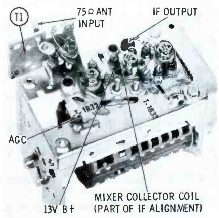
Fig. 6. Standard's transistor tuner used in Motorola Astronaut 19" TV.
