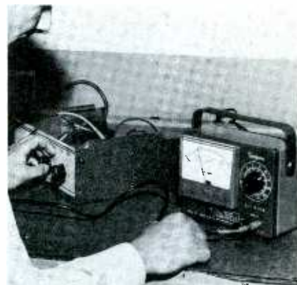
Fig. 4. New Simpson VTVM is geared for measuring small AC voltages.
