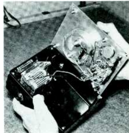
Fig. 2. The 109 has a sealed meter movement and three-cell power pack.
