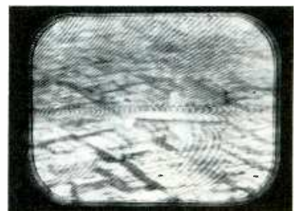
Fig. 5. "Herringbone" patterns usually indicate adjacent-channel interference.
