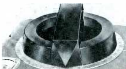
Fig. 8. Compact ferrite-core loop is often used in portable RDF equipment.
