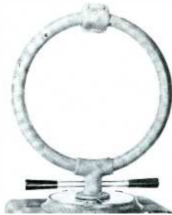
Fig. 7. Electrostatic shield on loop is broken by insulated collar at top.
