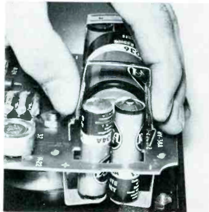
Fig. 6. Spring clips hold small batteries and serve as electrical contacts.
