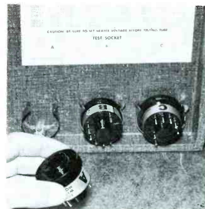
Fig. 6. Three socket adapters for different bases furnished with the 440.
