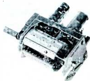
Fig. 3. Standard Coil GG Series turret tuner measures 2¼" x 2⅝" x 3⅝".
