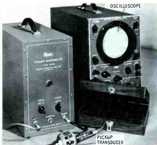
Fig. 8. Electronic micrometer, used with scope, is accurate within .0001".
