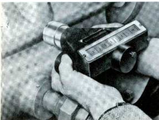
Fig. 2. Vibration analyzer for use in preventive maintenance of motors.
