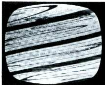
Fig. 1. Simple horizontal sync loss.
