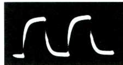
(B) Rounded leading edges (500 kc.)
