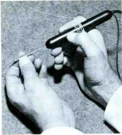
Fig. 9. Probe for the Craftscope has reversible tip for 1:1 and 10:1 inputs.
