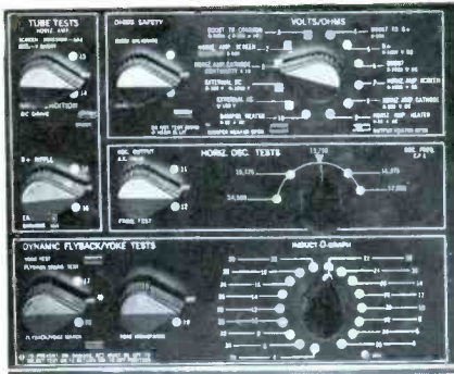
Fig 3. Model 250 switch positions follow a logical troubleshooting sequence.
