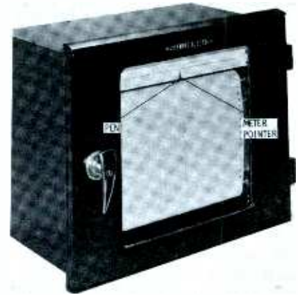
Fig. 5. Strip-chart device that records and corrects temperature variations.
