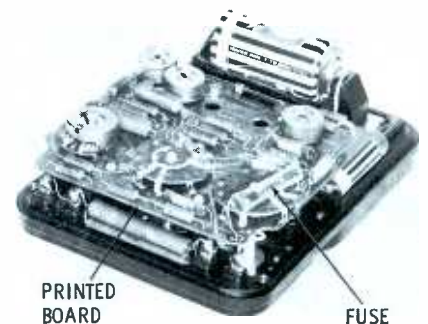
Fig. 8. Simpson 270 chassis comes out of case after removing only four screws.
